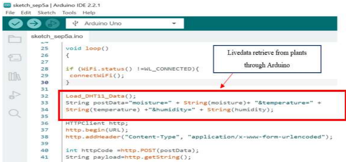
Figure 4. ESP32 connected and retrieved plants' live data
